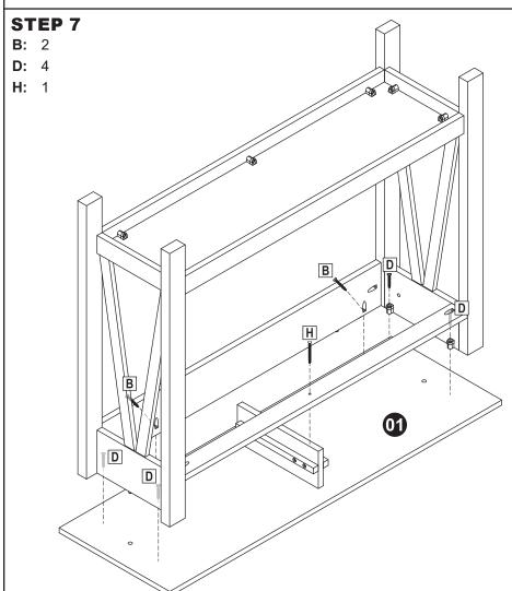
Align the assembled frame with the top.
