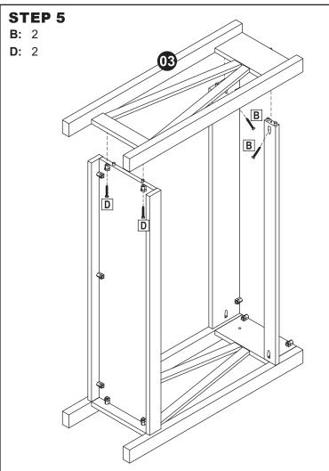
Secure Left Side Panel (03) using two M4.5mmx28mm Pan Screw (B) and two M4.5x25mm Pan Screws (D), as shown.
