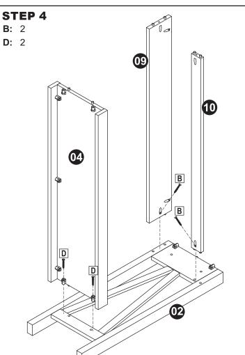
Secure Back Panel (09) to Right Side Panel (02) using one M4.5mmx28mm Pan Screw (B). Then, secure Front Crossbar (10) using one M4.5mmx28mm Pan Screw (B). Secure the shelf using two M4.5x25mm Pan Screws (D).
