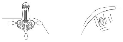
Step 3. If the tab on the foot is not sitting flush on the lug surface, you may insert either the rubber wedge shim or the steel shim to ensure better contact, a small gap will not affect the stability of the tub, tighten lock nut once you are satisfied with the fit of the tub foot.
