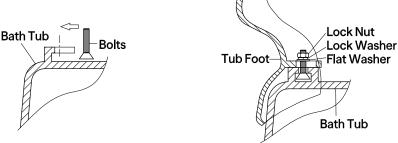
Step 2. Adjust foot for best fit, move the foot to ensure a good contact at all 3 points of the foot, both the tub lug and the tab on the foot have adjustment slots cut to allow horizontal and vertical movement and thus facilitate proper adjustment.
