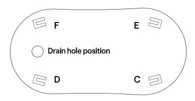
Letters marked beside the lugs on the bottom of tub
