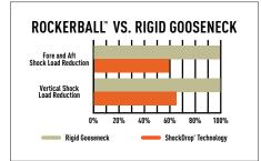
Cushioned isolator reduces rattling and vibration while the offset pin dampens vertical chucking and fore-to-aft motion during starts and stops, ultimately improving ride comfort and quality
