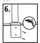
Use the provided self-tapping screws and a drill to secure rail mount into the vertical surface
