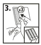
One at a time, adhere the Command strips to the bottom of the surface mount leaving the entire rounded and non-adhesive edge extending beyond the edge of the metal mount. This will allow for easy removal if necessary. Repeat this 2 times for the remaining Command strips
