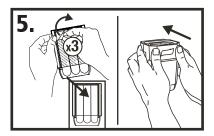
Remove BLACK liner from three Command Strips and place base on surface. Press firmly for 30 seconds.
