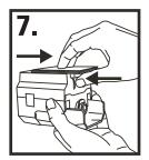
Press the release lever located on the bottom of the base; slide off the wall plate
