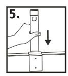
Place the mount against the surface in the desired location and firmly
