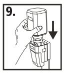
Load refill into the base with the PURELL label facing out making sure there is an audible click when the refill is in place
