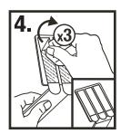
Peel the protective paper from the wall side of each command strip
