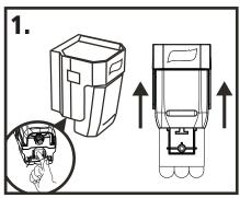
Depress release lever behind push bar and slide base off mount plate.
