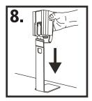
Slide base onto the surface mount making sure there is an audible click when the base is in place
