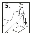
Place the mount against the surface in the desired location and firmly press
