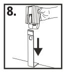
Slide base onto the rail mount making sure there is an audible click when the base is in place
