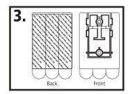
Remove RED liner from three Command® Strips and press each firmly on mount plate with tabs extending below edge as shown.
