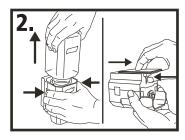
Remove refill by depressing right and left release buttons. Remove mount plate by depressing release lever behind push bar and sliding mount plate. Set refill and base aside.
