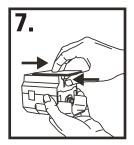
Press the release lever located in the bottom of the base and slide off the wall plate
