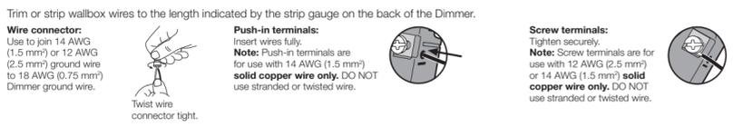
Wire connector: Use to join 14 AWG (1.5 mm) or 12 AWG (2.5 mm) ground wire to 18 AWG (0.75 mm) Dimmer ground wire. **Push-in terminals:** Insert wires fully. **Note:** Push-in terminals are for use with 14 AWG (1.5 mm) or 18 AWG (0.75 mm) **solid copper wire only**. DO NOT use stranded or twisted wire. **Screw terminals:** Tighten securely. **Note:** Screw terminals are for use with 12 AWG (2.5 mm) or 14 AWG (1.5 mm) **solid copper wire only**. DO NOT use stranded or twisted wire.
