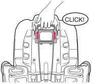
**3. Assemble the backrest.** Slide adjustment track into backrest assembly while squeezing handle. Make certain adjustment track can slide freely into different positions.
