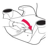
6. Install the backrest assembly. Position the base under the backrest assembly. Slide the backrest assembly onto the base. Make certain the backrest assembly locks into place with an audible click.
