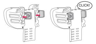
To install the Booster Inserts, line up the tabs to the slots at the rear of the backrest. Slide the Booster Inserts onto the backrest. Make certain the Booster Inserts lock into place with an audible click.
