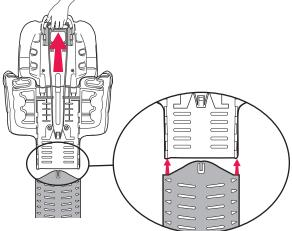
4. Attach the seat pad to the backrest assembly.
