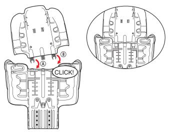
2. Install adjustment handle. Align tabs on adjustment handle with the slots on the back of the headrest. Press adjustment handle against the back of the headrest and slide upward until the tabs click into place.
