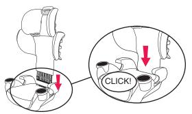
7. Check your work. Inspect the Booster Seat. Pull up on the headrest to make sure it is securely attached to the backrest. Make sure the seat pad is hooked into place. Pull on the backrest to make sure it is securely attached to the base. Repeat any assembly steps as necessary.
