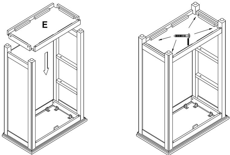
**Do not over tighten Bolts at this time. Assemble Loose.**
