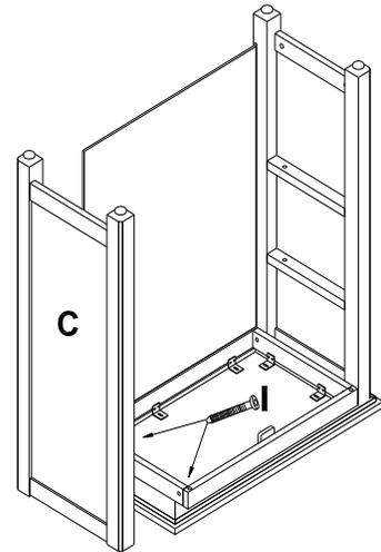
**Do not over tighten Bolts at this time. Assemble Loose.**
