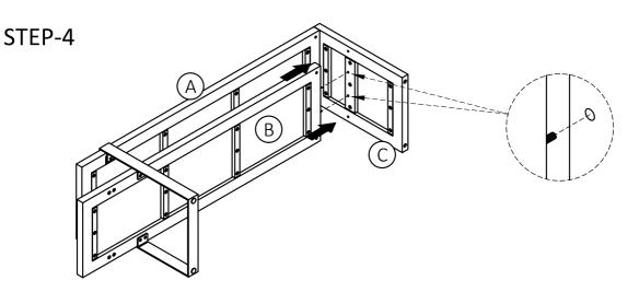
1. Align two guide holes on Side Panel (C) with two Wood Dowels on Shelf (B) and attach Shelf (B) to Side Panel (C).
