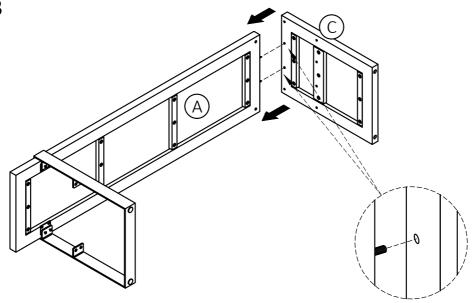
1. Align two guide holes on Side Panel © with two Wood Dowels on Top (A) and attach Side Panel © to Top (A).
