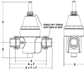
ABOVE VALVE SHOWN WITH SINGLE NPT UNION CONNECTION ON INLET VALVES MAY BE ORDERED WITH 0, 1, OR 2 UNION CONNECTIONS USING ANY COMBINATION OF NPT, SOLDER. PEX, QUICK CONNECT, CEF (F1960), PRESS OR CPVC CONNECTIONS REQUIRED
