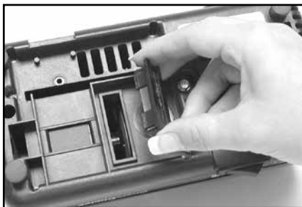
Figure 18. Removing cover under base to clean out metal dust (See Normal Maintenance section).
