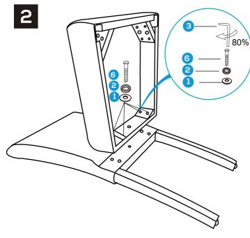
Secure both corner holes of the seat pad to the chair back by using LONGER SCREWS (6) with washers (#2,1).
