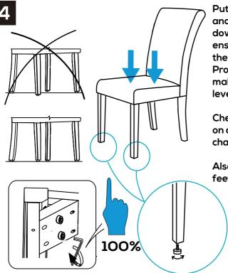
Put chair in the upright position and SIT ON THE CHAIR to press downwards on the seat pad ensuring that all 4 feet touch the ground and chair is leveled. Proceed to tighten all screws making sure the chair remains level when tightening.
