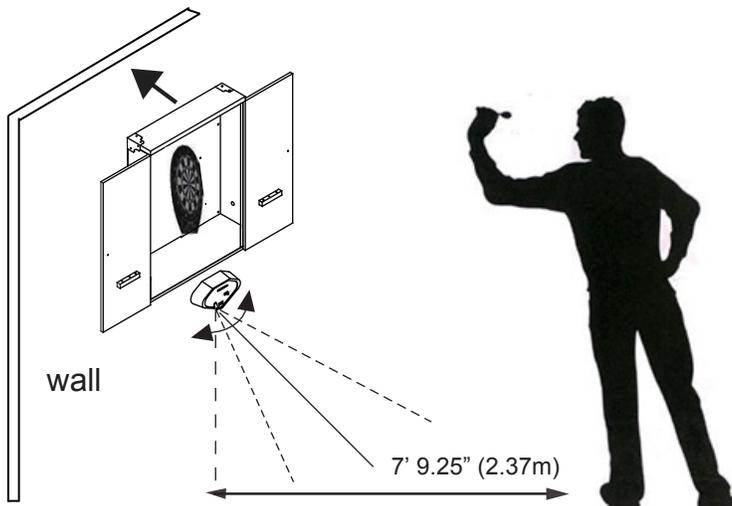
Adjust Laser Line to 7' 9-1/4" (2.37m) from face of dartboard
