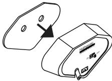
1. Mount your dartboard or dart cabinet. With one hand place the Laser Dart Line on the wall or cabinet directly below and centered on the dartboard. With your other hand level the Laser Dart Line.
