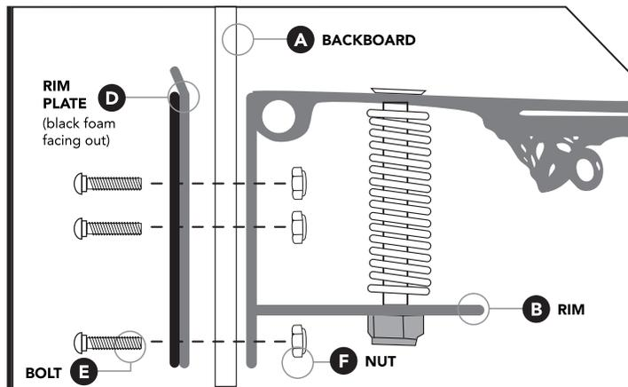
Align the holes on the Rim Plate (D) with the Backboard (A) fitting the Rim Plate against the back of the Backboard. Using the Bolts (E), attach the Rim (B) to the backboard making sure the square head of the screw fits securely to the square cut out on Rim Plate. Tighten each Nut (F) with a Wrench (G) to secure the Rim to the Backboard.
