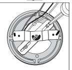
4. Adjust the crossbar fixture screws and tighten the center swivel screws. Before installing the fixture canopy, add silicone sealant between the front of the round plate and fixture canopy. Insert the fixture canopy holes through fixture mounting screws (Fig D).
