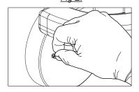
2. Before installing the round plate, add silicone sealant between the rear of the round plate and the J-box. Pull the power supply wires through the round plate and install the round plate along with crossbar, onto the J -box with the screws provided (Fig B).
