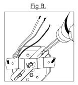
Adjust the crossbar fixture screws and tighten the center swivel screws. Insert the canopy holes through fixture mounting screws (Fig D).
