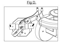
6. Caulk between the light fixture and the wall surface with a silicone sealant (not included).
