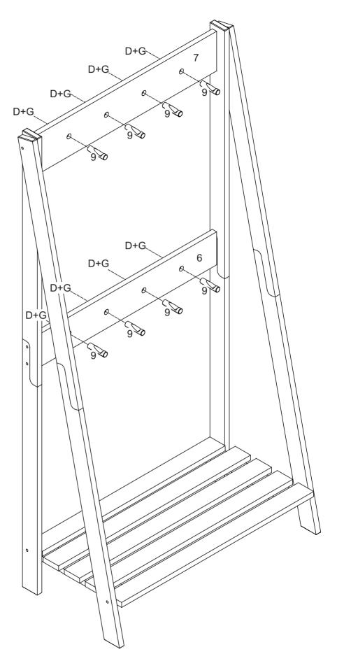
Secure pegs (9) to parts (6,7) using screw (G) and hex key (D).
