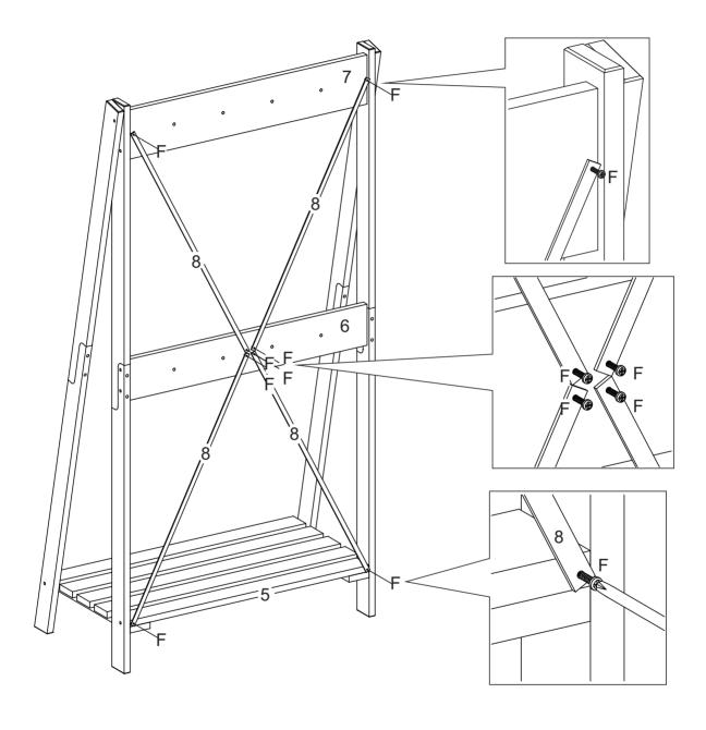
Attach part (8) to parts (5,6,7) using screw (F) and Philips Screwdriver.
