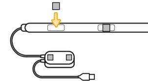
3. Apply 2 pieces of double-sided mounting tape to the back of the crib light and 2 pieces to the back of the control unit.
