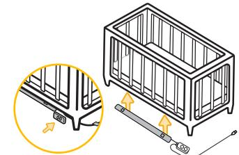
4. Adhere the crib light to the underside of the crib.
