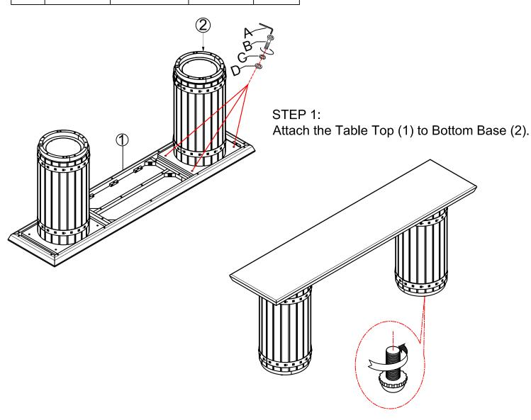
Adjust leveler if needed to level console on uneven floor.
