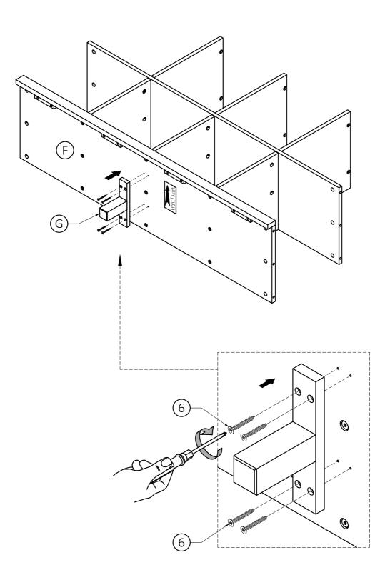
1. Align Bottom Support Leg (G) with pre-drilled holes on back of Bottom Shelf (F). Use Phillips Screwdriver to tighten four Phillips Screws (6).
