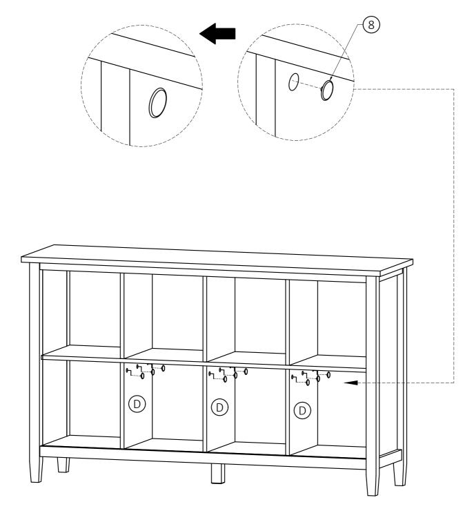
1. Insert Plastic Caps (8) into holes Cam Locks on Dividers (D).
