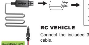
Connect the included 3.7V battery to the charging cable.
