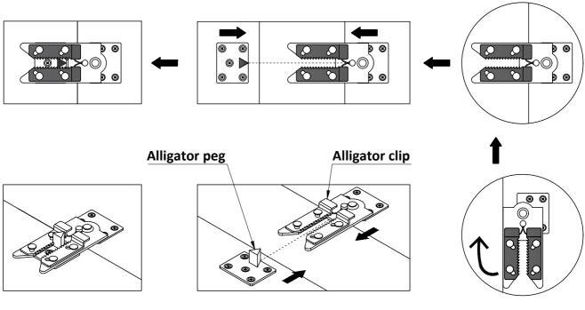
Rotate the connector clip 90 degrees.
