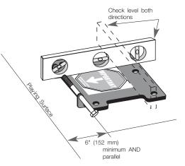
Step 6: **Position 6" ground anchor (Item G2660) in center of hole** with hinge side toward and parallel with playing surface. Using a level, ensure the anchor is level front-to-back and left-to-right. All edges of the ground anchor must be 6" (15.2 cm) away from all sides of hole and the top of the ground anchor within a range of 1"- 3" (25-75 mm) above the level of the playing surface.
