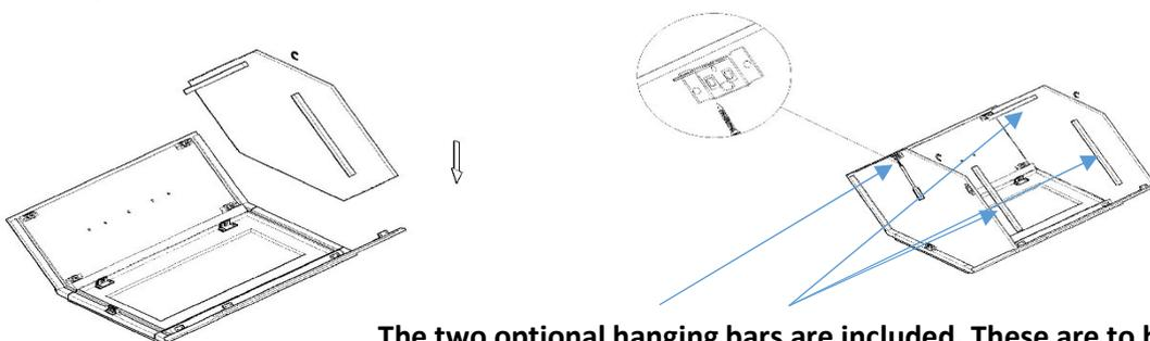
The two optional hanging bars are included. These are to be installed at the top and bottom of the inside of the cabinet prior to mount to the wall. The Larger screws(M 2 3/8") are needed.
