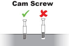
Use a screwdriver to tighten the cam screw until the shoulder is flush with the panel. Do not over-tighten or under-tighten.
