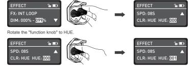
Rotate the "dimmer knob" to set the HUE parameters.
