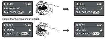
Rotate the "dimmer knob" to set the CCT parameters.
