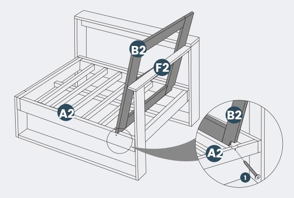
Attach **Part B2 Backrest** to **Part G2 Chair Right Arm** and **Part A2 Chair Seat** with 1 pc of **Hardware #2 Screw**.
