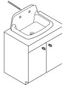
Set the sink at the desired place and mark a horizontal leveled line at where the top of the backsplash will be situated, remove the sink, place template on the wall and align the leveled line, making sure that the sink front is parallel to the front of the counter. Be sure the sink is properly centered, both front to back and side to side.
