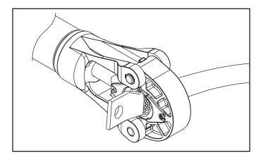
For a UL or cUL classified crimp, complete the number of crimps specified under "Connector Selection". 5. For a single crimp, position the connector so the crimp will be located at the center of the barrel.
