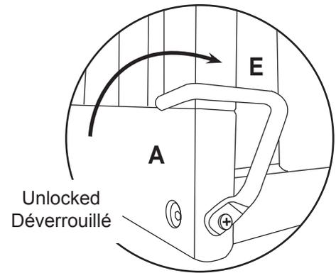
\* **Allow the cradle to rock:** rotate the rocking stop (E) clockwise to unlock.
