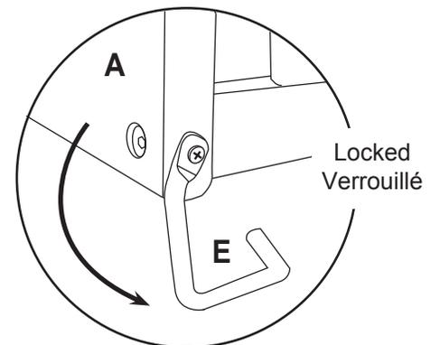
\* **Stop rocking:** rotate the rocking stop (E) counter clockwise to lock.
