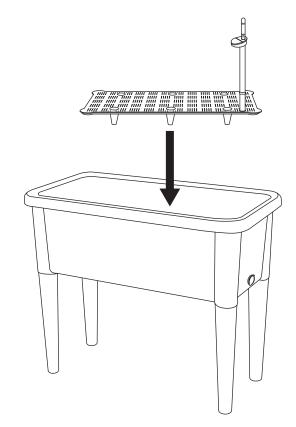
Place the grid with the watering tube into the planter box.
