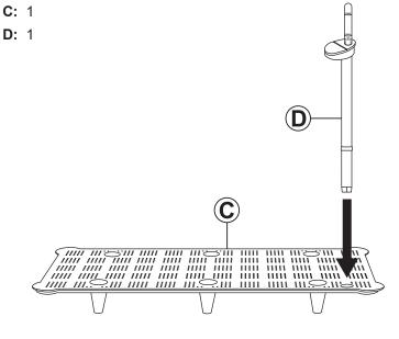
Insert the bottom of Watering Tube (D) into Grid (C) as shown.
