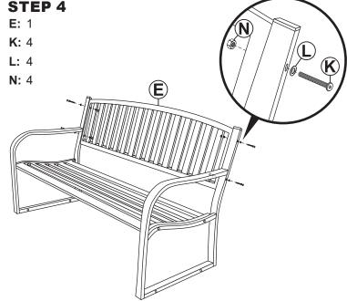
Secure Backrest (E) to the top of the arm panels using four M6x70mm Bolts (K), Flat Washers (L), and Nuts (N).
