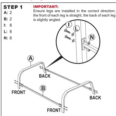
Loosely fasten two Legs (A) to two Stretchers (B) using four M6x35mm Bolts (I), Flat Washers (L), and Nuts (N).
