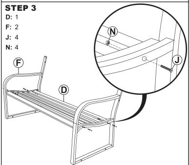
Secure two Arm Panels (F) to the middle of Seat (D) using four M6x50mm Bolts (J), and Nuts (N).
