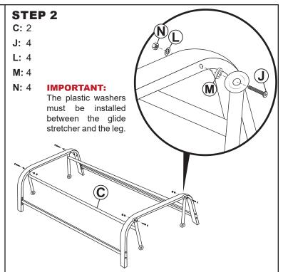
Align the short side of Glide Stretcher (C) with the outside of the legs and loosely secure using two M6x50mm Bolts (J), Flat Washers (L), Plastic Washer (M), and Nuts (N), as shown.
