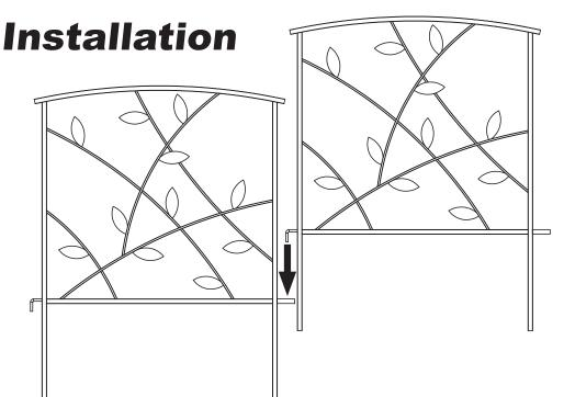
Insert the first fence panel into the ground by carefully pushing the legs into the soil.
