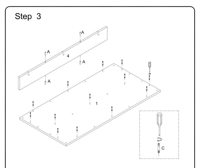
Insert wooden dowel (A) into part (4), then secure cam bolt (C) into part (1) with Philips head screwdriver as per diagram.
