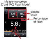
About the Analog Scale Details Measuring value (f-stop)
