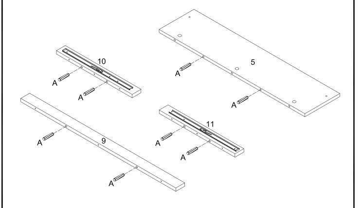
(EN) Insert wooden dowels (A) into back panel (5) and drawer panels (9)(10)(11).
