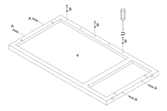
(EN) Insert wooden dowels (A) and bolts (B) into the table top.
