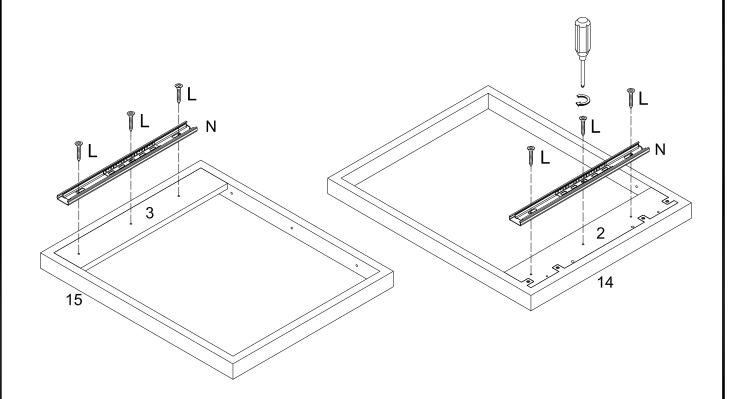
(EN) Secure screw (L) to the tray arm of keyboard tray slider (N) to the side panel (2,3).
