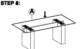
**POSITION PEDESTALS UNDER GLASS TOP TO PROVIDE MAXIMUM SUPPORT DURING USE**
