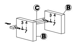
LAY BOTH PEDESTAL BASES ON SIDE TO ATTACH STRETCHER
