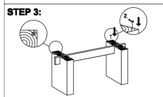
**BUMPERS SHOULD BE APPLIED TO BOTH PEDESTALS TO** PREVENT GLASS FROM MOVING
