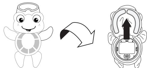
**2** Use a Phillips screwdriver to loosen the screw that secures the battery cover.
