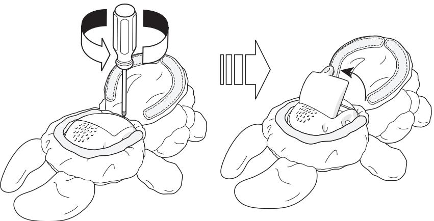
**3** Install (3) size AAA/LR03 (1.5 V) batteries, observing the polarity markings embossed on the bottom of the compartment.
