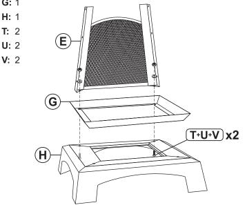
Place Base Panel (G) on Leg Panel (H) and fasten Back Screen (E) using two Bolts (T), Washers (U), and Nuts (V).
