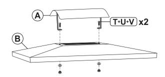
Fasten Cap (A) to Top (B) using two Bolts (T), Washers (U), and Nuts (V).
