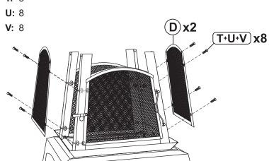
Secure each Side Screen (D) using four Bolts (T), Washers (U), and Nuts (V).
