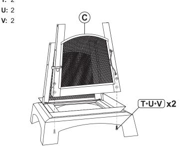
Fasten Front Screen (C) using two Bolts (T), Washers (U), and Nuts (V), as shown.
