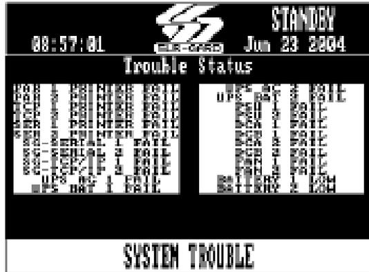
When a trouble is present in the SG-System III the message '**SYSTEM TROUBLE**' will displayed at the bottom of the screen
