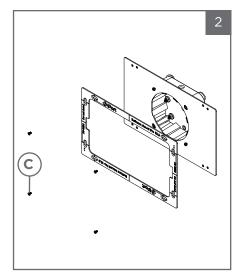
Use the 4 provided #6-32 x 1/4 IN Flat Head screws to mount the surface mount bracket (found on the back of the Surface Mount Bezel (e) sold seperate) to the Vesa mounting bracket (a).
