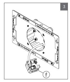
Insert a cat5/6 cable through the 5/8 IN hole in the side of the VESA Box and connect the iPort Splitter (f) (Sold Seperatly)
