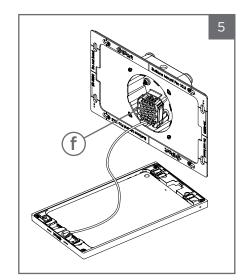
Connect the appropriate power source identified in the Power and Wiring Guide (found in PoE splitter (f) box). Place the PoE splitter into the VESA mount box with the iPort logo facing out.
