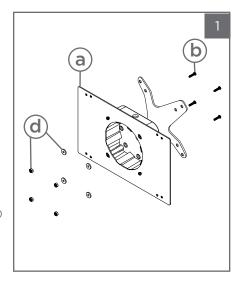
Take the 4 provided #6-32 x 5/8 IN Pan Head screws (b) along with the provided washers and nuts (d) and attach the VESA mounting bracket (a) into your desired Vesa Mount as shown.
