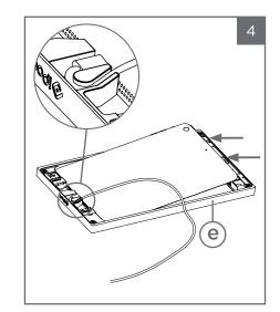
Plug in the iPad's lightning to USB cable directly into the iPad. Position the iPad facedown into the bezel (e) with the iPad cable on the left. Carefully wrap the iPad cable around the metal loop located on the bezel. To lock the iPad in place, use a flat head screwdriver to deploy the second and third toggles located on the right side of the Surface Mount bezel. The first top-right toggle is a power button extension.
