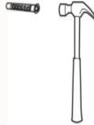
Hammer the expansion screw (4) into the wall with a hammer.
