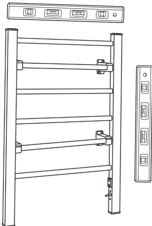
Fix 4 Wall mounting brackets on the shelf, then place the shelf lightly on the wall, and adjust the position with a level meter. Mark the position of the screw hole with a pencil.
