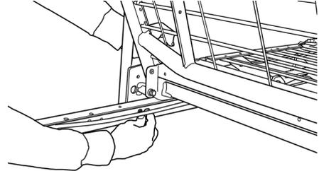
4. Place additional hex bolt and spring washer through the bottom hole.
