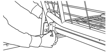
3. Place 5/16"-18 x 3/4" Hex Bolts with Spring Lock Washer through the hole in the frame and hand tighten.
