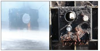
See how the barrier stands tough against hose stream and survives fire. Watch the fire test video at www.3M.com/Firestop
