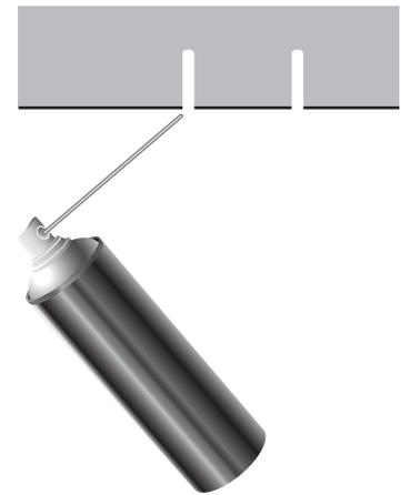
Clean loose debris from the pilot holes using a blower, canned air or a vacuum.
