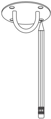
Position the round eye pad on the hanging surface, then mark the positions for the four holes.
