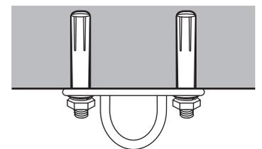
Position the round eye pad over the expansion bolts. Place the flat washer then split washer on the bolt, then hand-tighten the nut. Fully tighten all hardware with a wrench.
