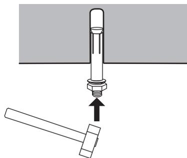
If installing into concrete/brick, tap in the expansion bolts. Expand them enough to hold in place by tightening the nuts, **do not fully tighten yet!**
