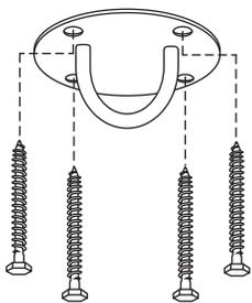
If installing into wood, position the round eye pad over the pilot holes and drive the screws into the pilot holes.
