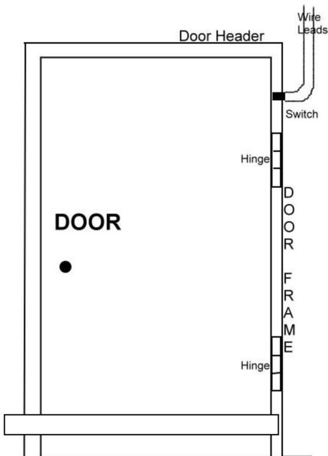
Drill 3/4" hole ON HINGE SIDE of window or door frame to mount switch\*
