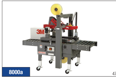
8000a 47 3M-Matic™ Side Belt Adjustable Case Sealer 8000a is an adjustable side belt drive case sealer. Seals up to 40 cases per minute, using tape widths from 36mm to 48mm, and also 72mm tape.
