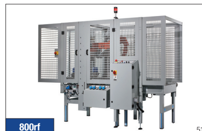
800rf 51 3M-Matic™ Case Sealer 800rf Type 40800 is a fully automatic random size case sealer that automatically adjusts for various case sizes and folds the top minor and major flaps up to 10 cases per minute. Using tape widths from 36mm to 48mm tape widths.
