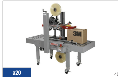
a20 40 3M-Matic™ Adjustable Case Sealer a20 is an adjustable bottom belt drive case sealer to dependably seal uniform cases at up to 30 per minute.
