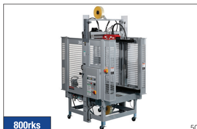
800rks 50 3M-Matic™ Case Sealer 800rks is a random king size case sealer that automatically adjusts for case height and width and is capable of sealing up to 10 cases per minute, using tape widths from 48mm to 72mm wide.
