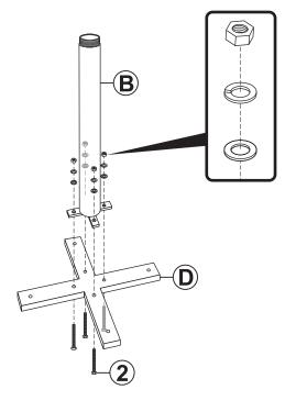
Firmly secure Crossbar (D) to Upper Pedestal (B) using four M8x40mm Bolt Sets (2).
