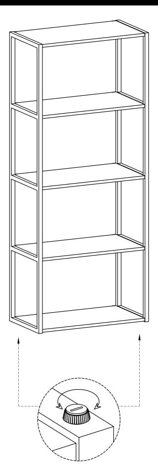
Note: Levelers on bottom of legs can be adjusted if floor is uneven.
