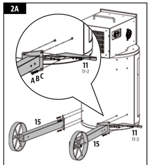
pre-drilled holes. Repeat installation for second leg with wheel (front side), but also install one front shelf support using the same hardware. Note illustration 2A for guidance.
