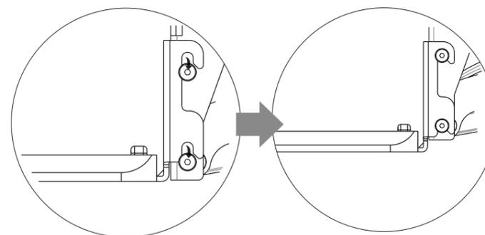
**c** Press the two buttons when to release the keyboard tray
