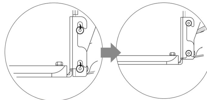
**c** Press the two buttons when to release the keyboard tray
