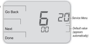
In Service Menu 620, press ▲ / ▼ to select option "01" to enable fan output (see Fig. 13).
